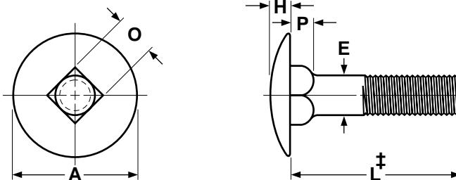
†Length of a step bolt is measured from the underhead bearing surface to the extreme end of the bolt.
